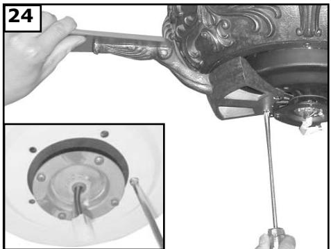
Remove the shipping stabilizer plate and throw away (see insert). The screws, washers and motor pads are pre-installed to the blade holders. Attach blade assembly to motor and tighten screws securely.
